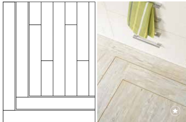
Straight laid plank with tramline strip perimeter (tramline planks can be supplied in bespoke width). Design ref: 507
